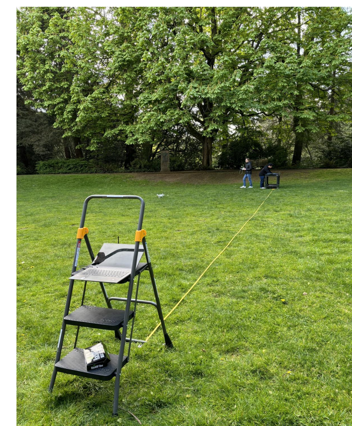
Above: (Left) TX antenna, 916-CW-RCL-SMA Monopole Antenna with Ground Plane and (Right) RX antenna, RFSPACE TSA400 Antenna with Ground Plane.
