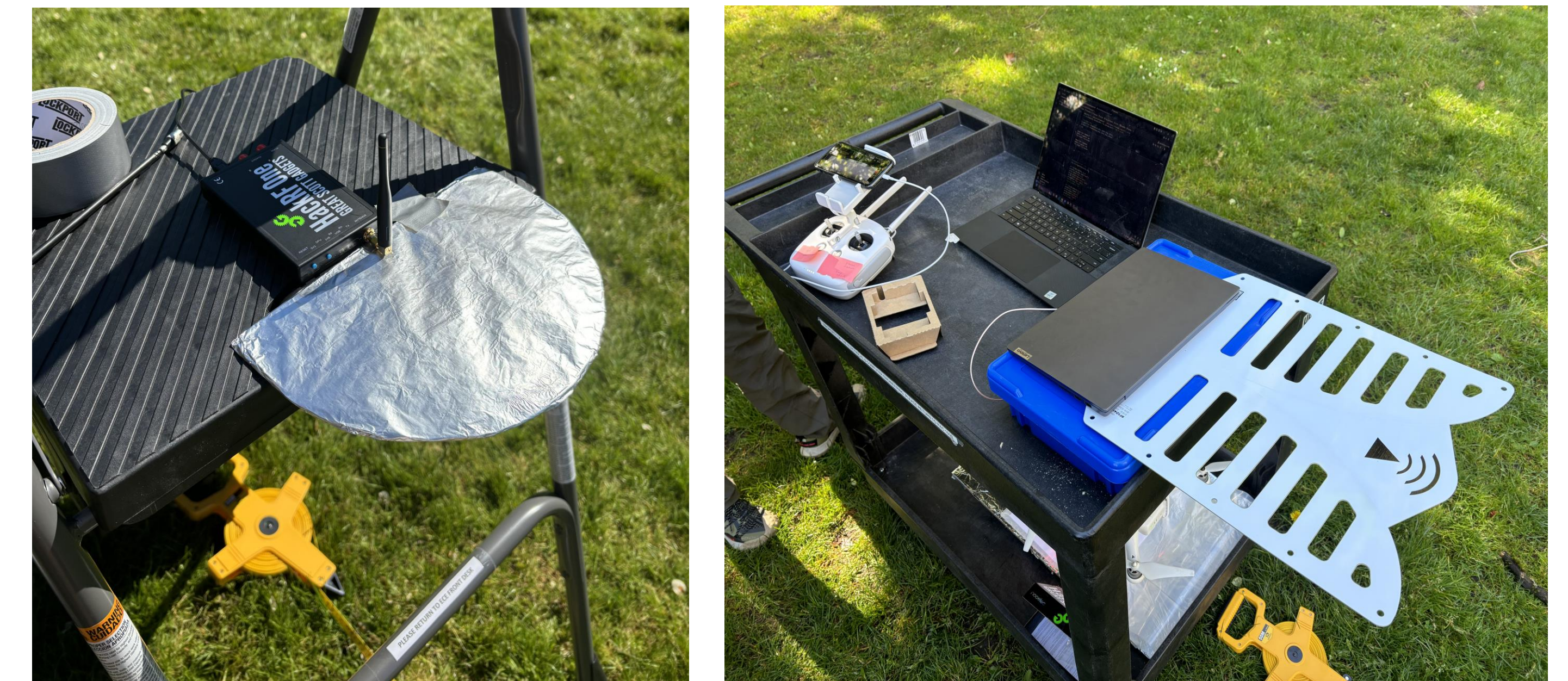
Above: (Left) TX antenna, 916-CW-RCL-SMA Monopole Antenna with Ground Plane and (Right) RX antenna, RFSPACE TSA400 Antenna with Ground Plane.
